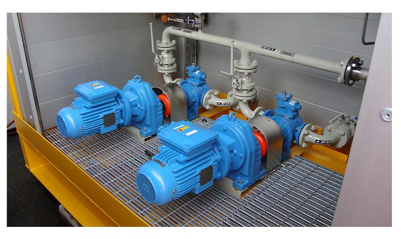
The Imenco aviation pump unit is a key unit in all our helicopter refuelling systems
